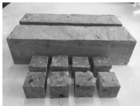
Fig. 3 Specimens for abrasion testing
