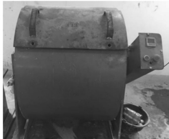
Fig. 2 Los Angeles machine for abrasion test
